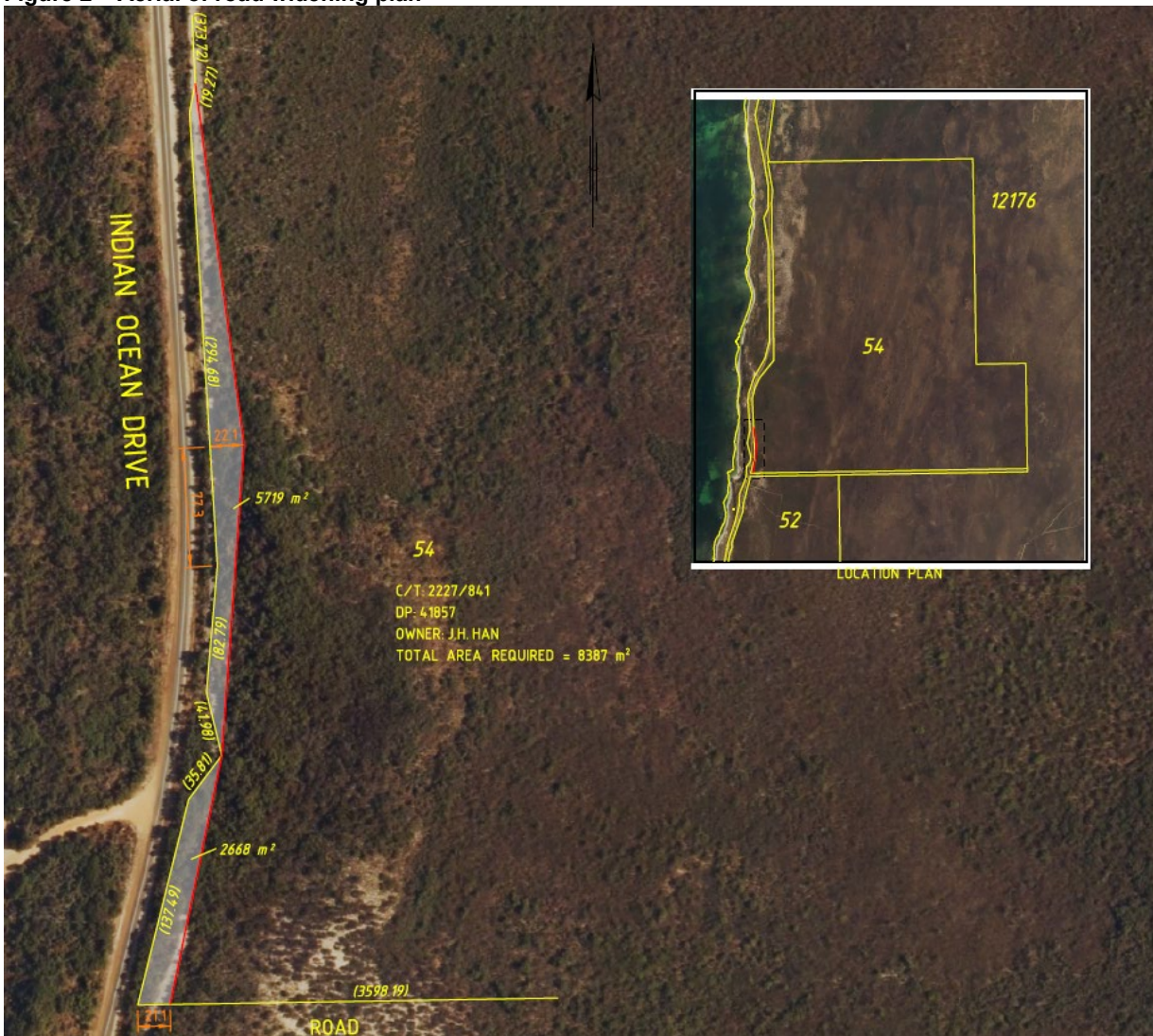
Figure 2 – Aerial of road widening plan
